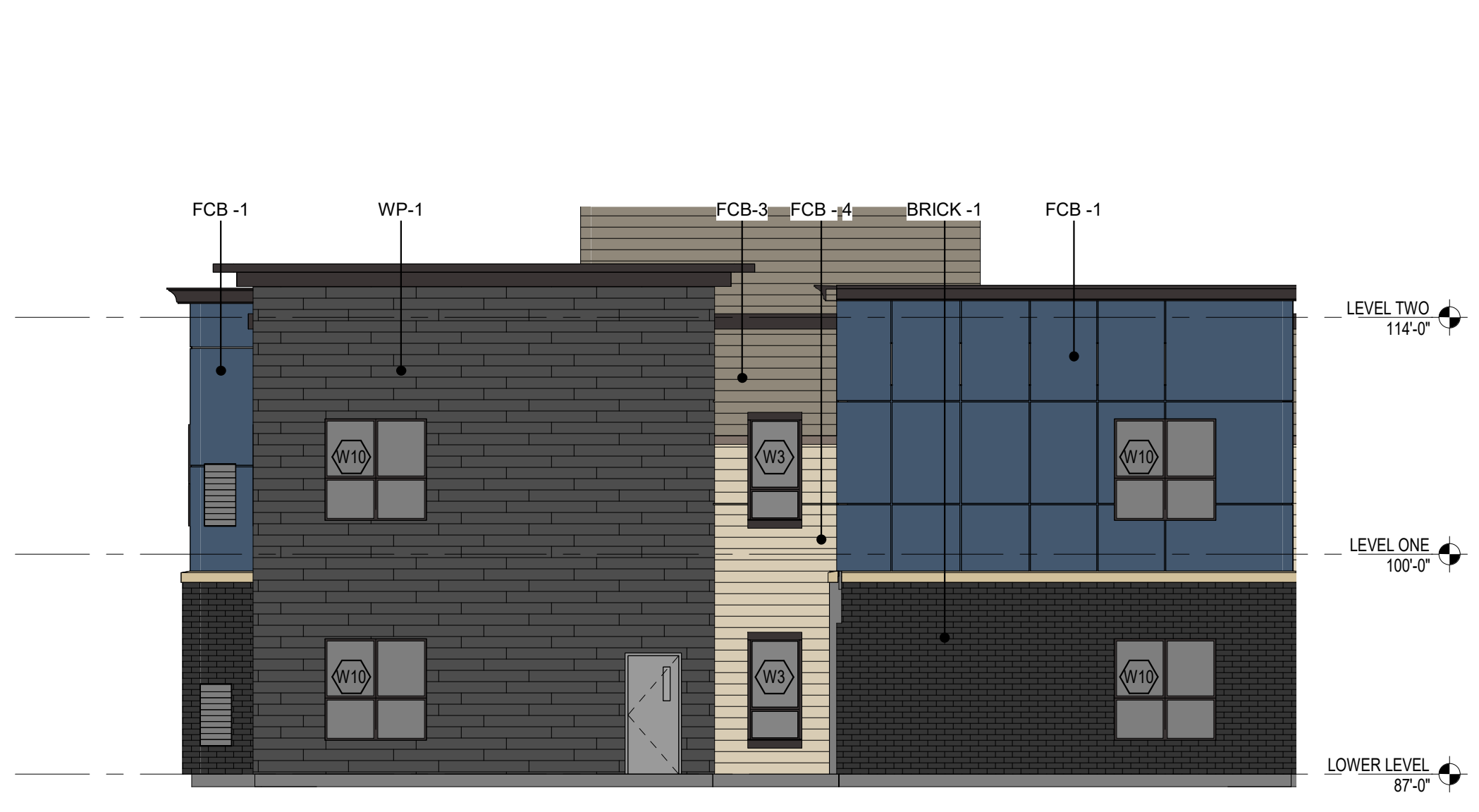
2 A3.4 AREA D - ASSISTED SOUTH ELEVATION 2 1/8" = 1'-0"
