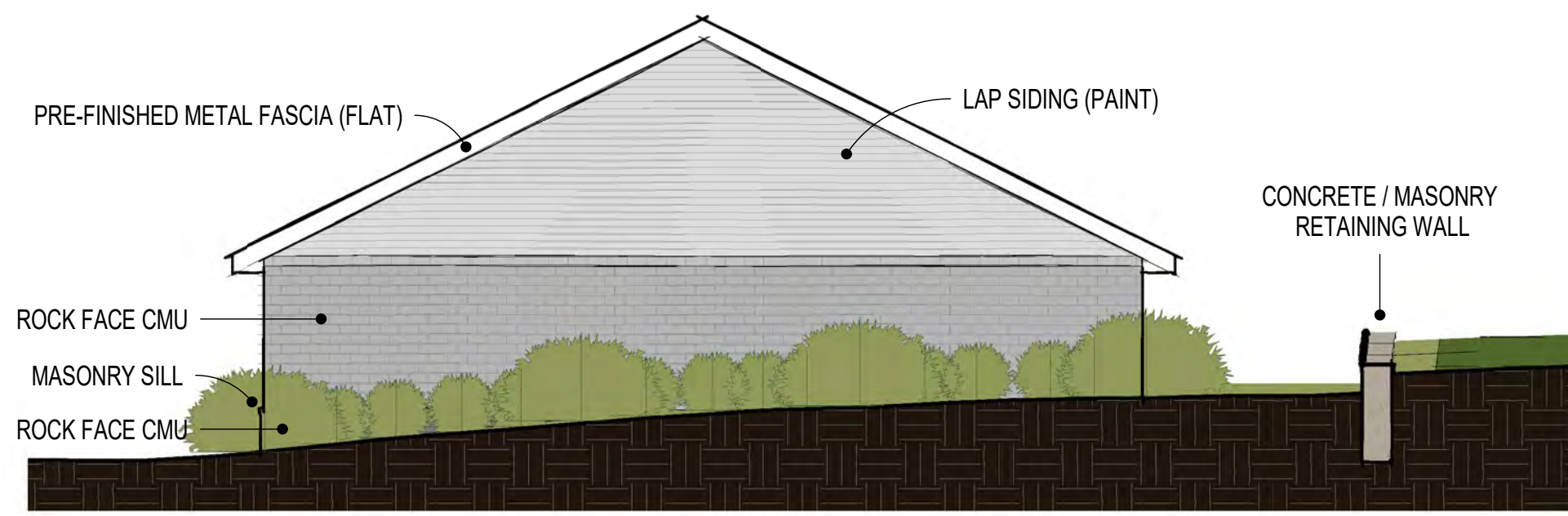
4 WEST ELEVATION - BUILDING "D"
