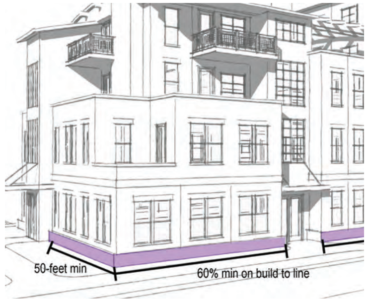
Diagram of building frontage requirements for primary street and corner lot frontage.
